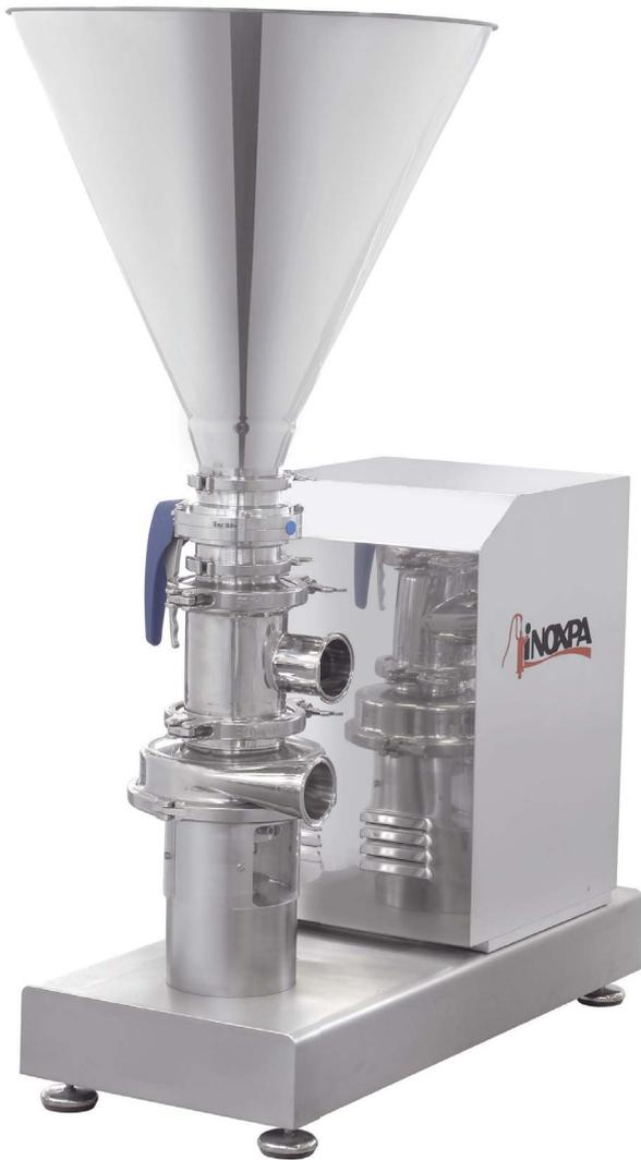
It is important to keep low pressure at the suction and at the discharge sides of the blender. Avoid cavitation. Thus a feeding pump must be provided only for the applications that really require it (considerable pressure drops at the suction side, high viscosity products, etc.), please, keep in mind that the suction capacity will decrease.
